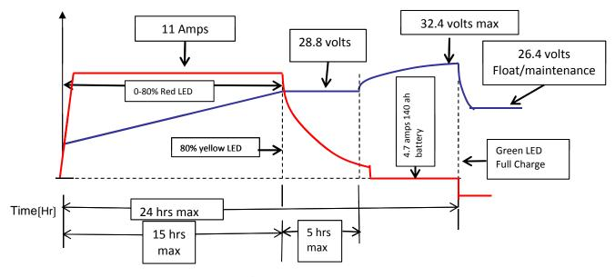
957760 and 957761 Setting # 2 Charging curve for wet 140 AH batteries
